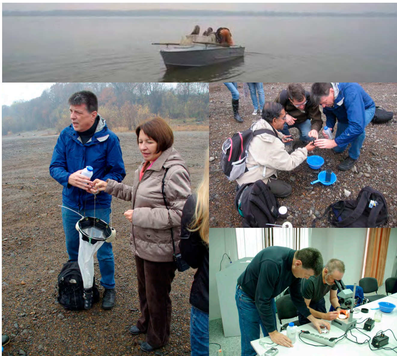
A field trip to the Amur River near Khabarovsk on October 15, 2011, provided an opportunity for some of the workshop participants to conduct surface tows for microplastics from a small craft. Shown here clockwise, starting at top is the sampling platform, participants decanting microplastic samples from the plankton net on shore, workshop members examining samples using a dissecting microscope in the laboratory of the Khabarovsk Branch of Pacific Research Fisheries Centre, Russian Federal Agency on Fisheries, and Drs. Joel Baker and Olga Lukyanova with 330 \mu\text{m} mesh plankton net prior to deployment. Photos by A. Subramanian, P.S. Ross and O. Lukyanova.
