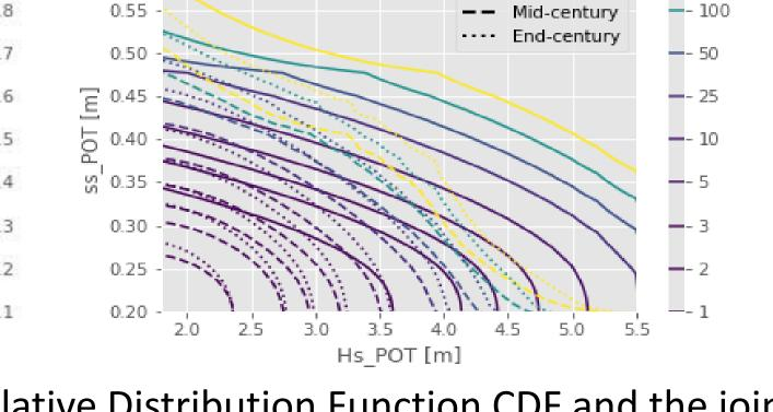
The two figures show the joint Cumulative Distribution Function CDF and the joint Return Period RT respectively of extreme events of wind waves and storm surge in one of the studied locations. For each pair of simultaneous extreme events, it is possible to estimate the probability of occurrence and the return time.
