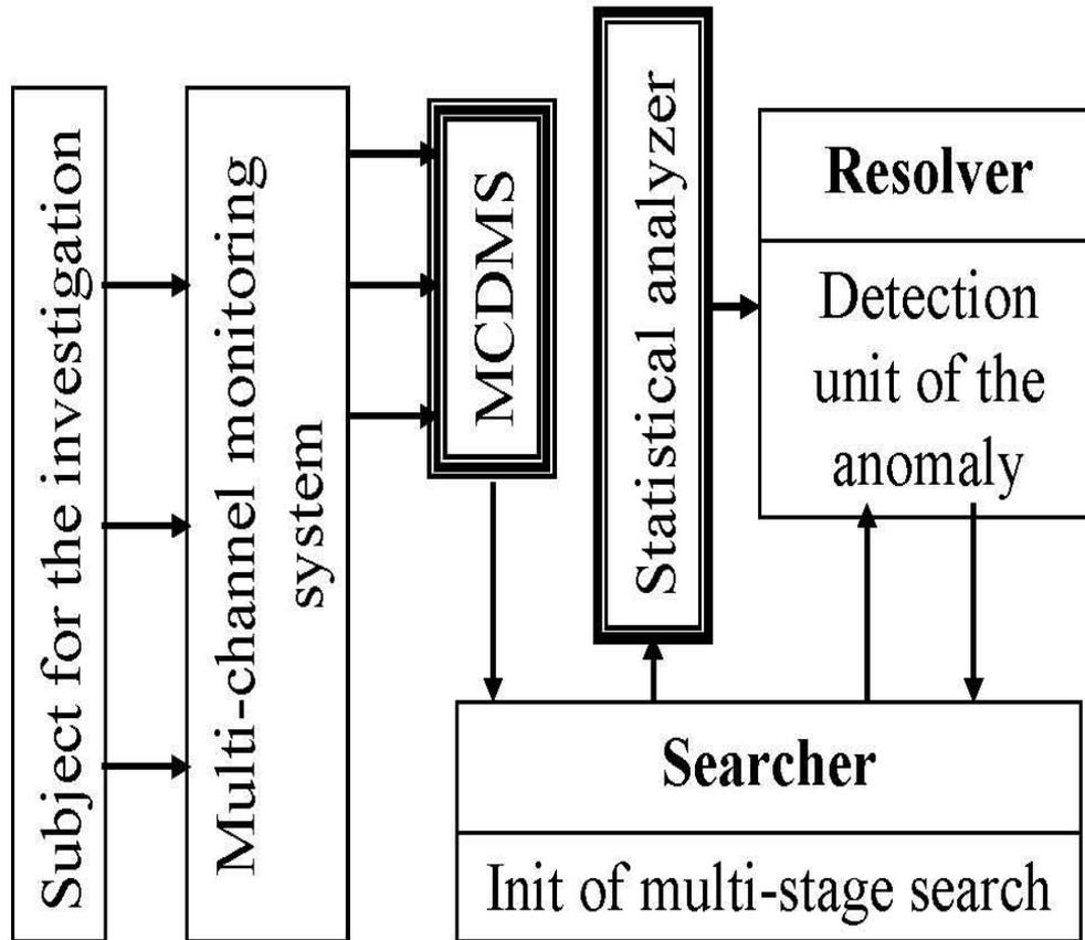
Searcher analyses values of indicator and localizes possible dangerous deviations forming their statistics on the base of which resolver makes a decision about the origin of dangerous changes in the studied system or process.
