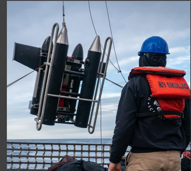
In Situ Ichthyoplankton Imaging system (ISIIS)
