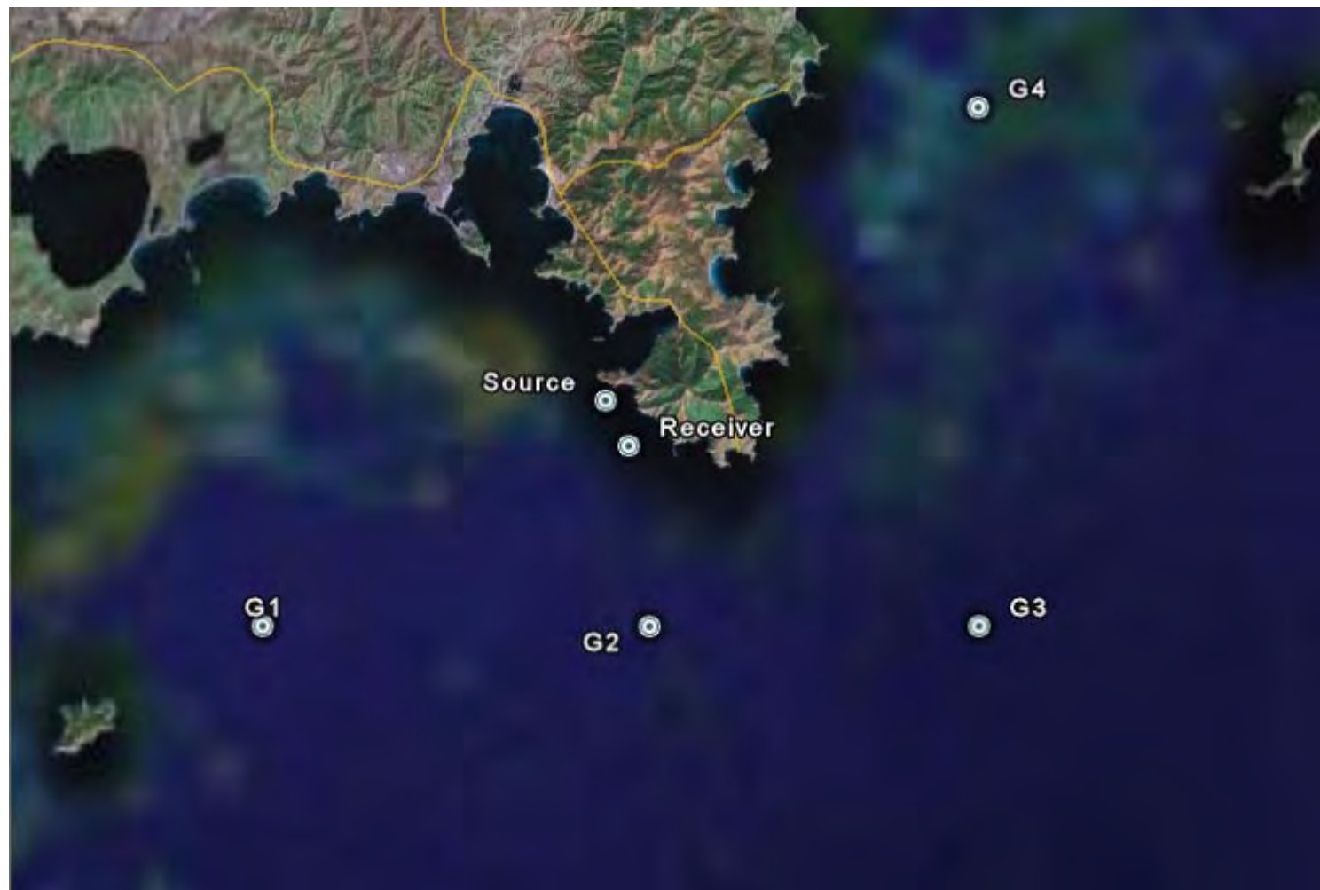
The sea chart of the acoustic monitoring experiments of hydrophysical characteristics conducted in the East/Japan Sea shelf zone. (S – source; R – receiver; G1-G4 - points of hydrological measurements)
