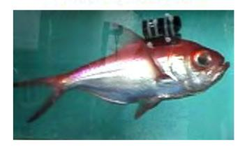
Acceleration data-logger D2GT in neutral buoyancy attached to alfonsino
