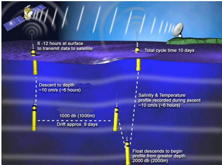
Iridium telemetry allows high-resolution (1-2 dbar), multi-parameter data transmission and two-way communication.
