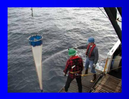
The net is a 0.5m diameter ring net, with 202µm mesh, towed vertically from a maximum of 100m (or 5m off the bottom) to the surface.
