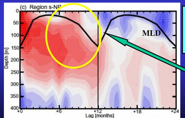
Lag correlation coefficients between anomalies of winter SST and the subsurface layer temperature in the NPSTMW formation area.
